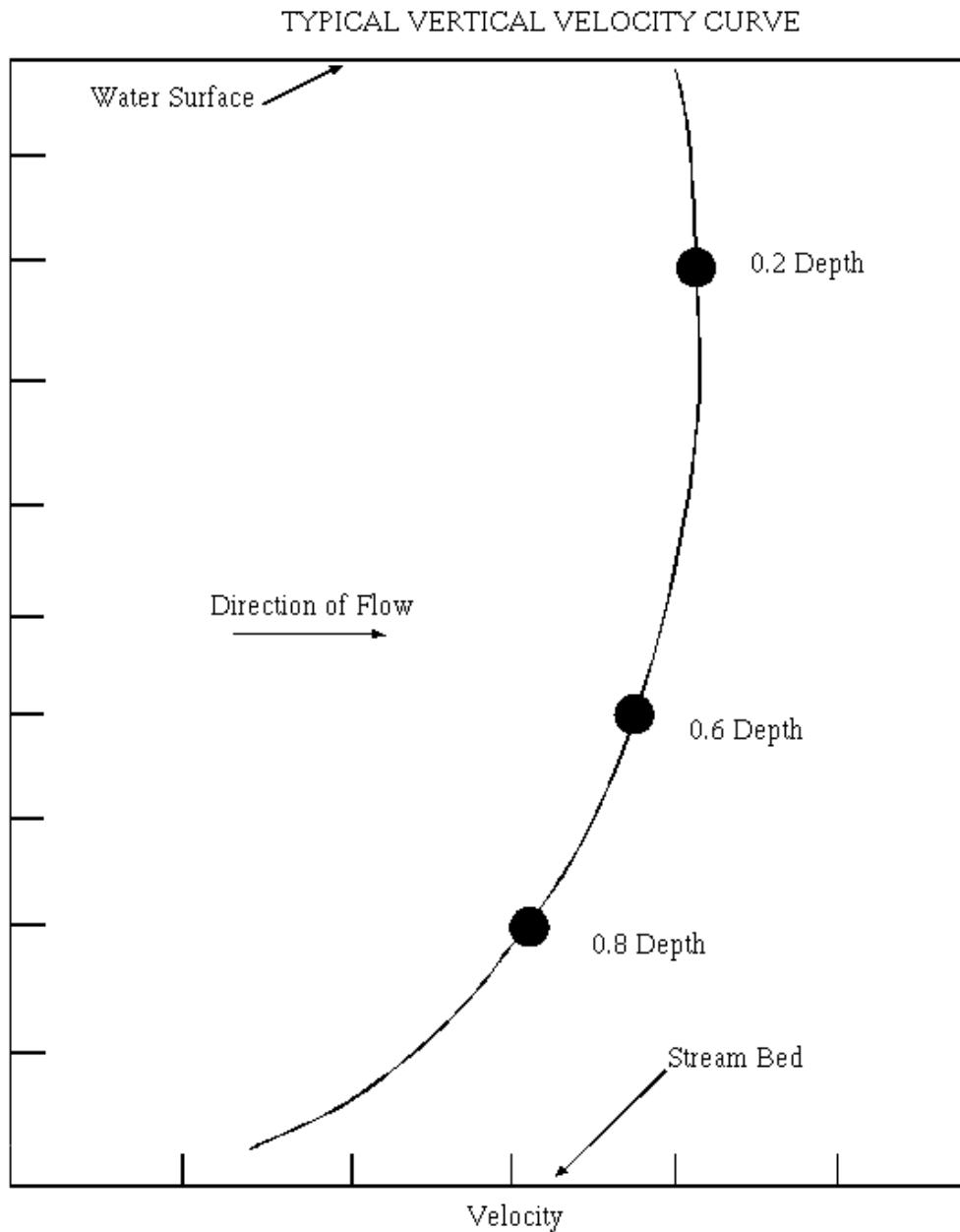
**Figure D-1. Example of typical vertical velocity curve.**
