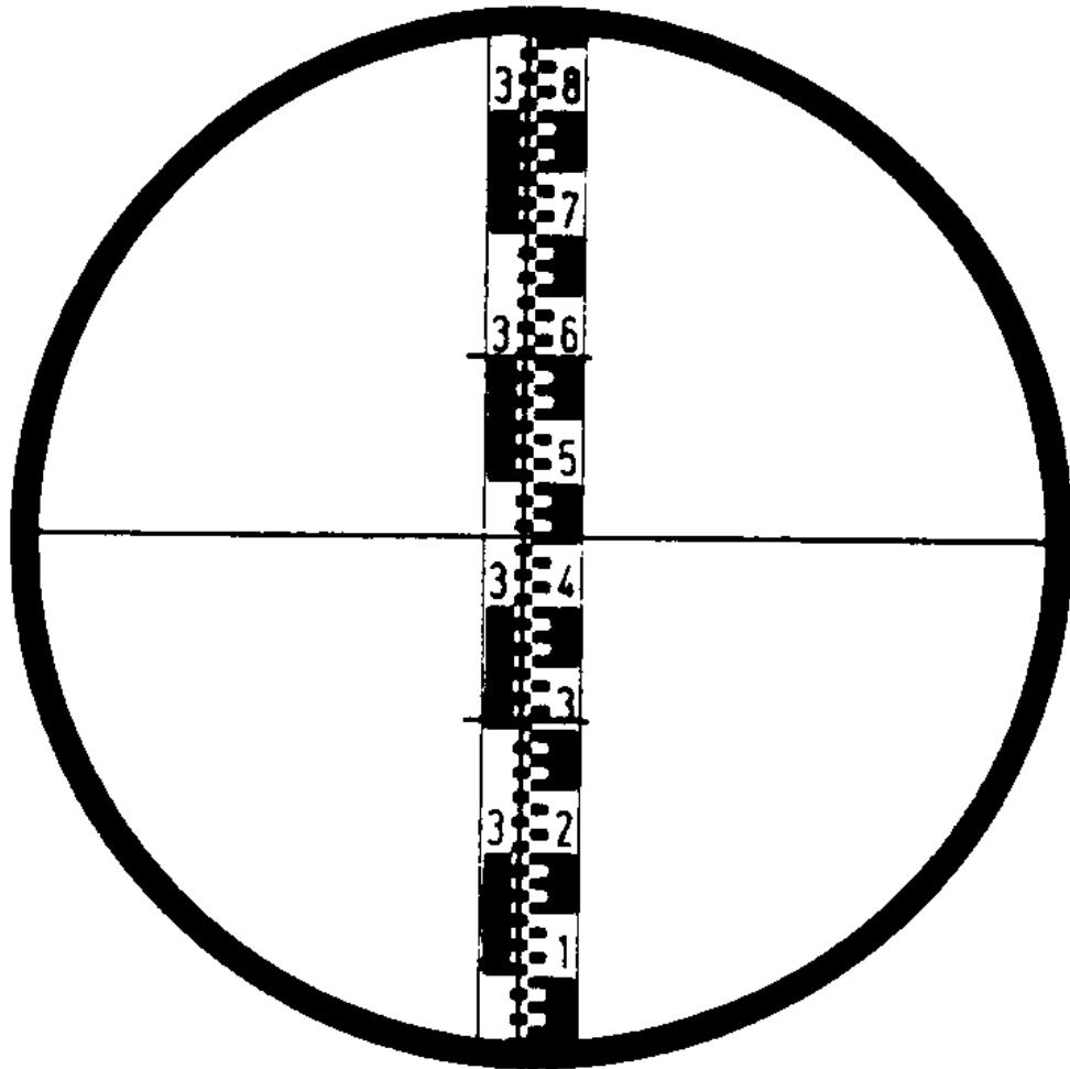
**Figure E-3. Reading the rod height 3.456 m, distance 29.2 m,** (Source: Automatic Level, Wild NAO, Instructions for Use, Manual G2 106e - IX.80, p.9).
