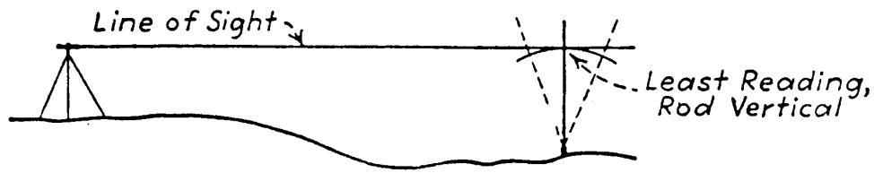
**Figure E-2. Positioning the rod.**
