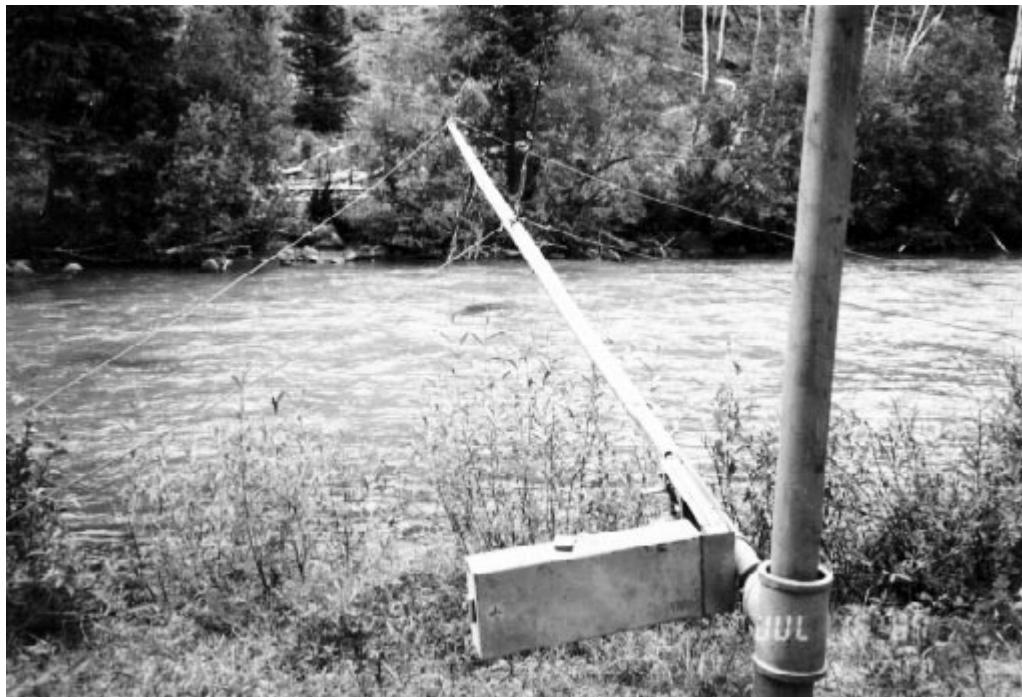
**Figure B-13.** Boom wire weight gauge.
