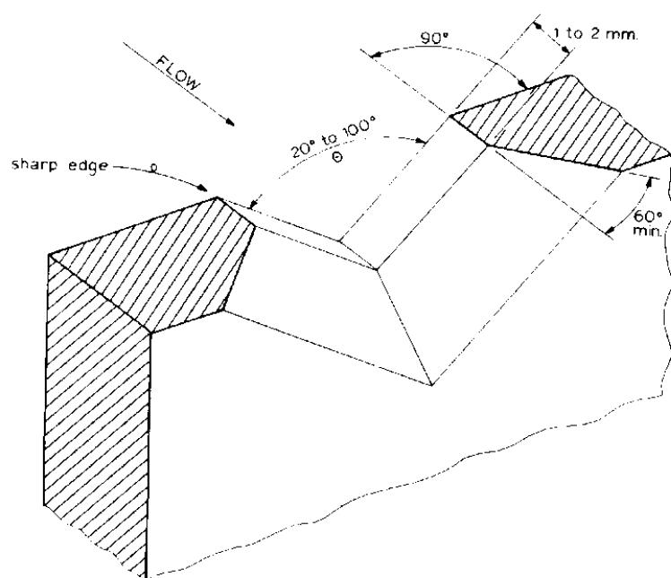
**Figure G-2. Top - V-notch sharp-crested weir. Bottom - Enlarged view of V-notch.****Table G-2. Comparison of two selected rated structures.**
