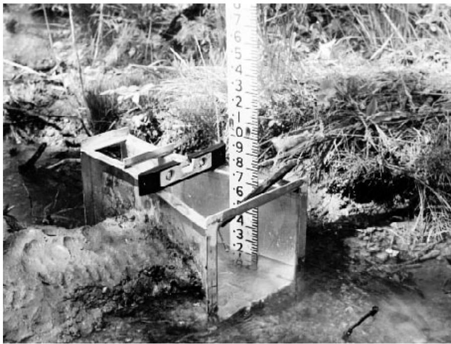
**Figure B-5. Three-inch Montana flume set in a mud dam.**
