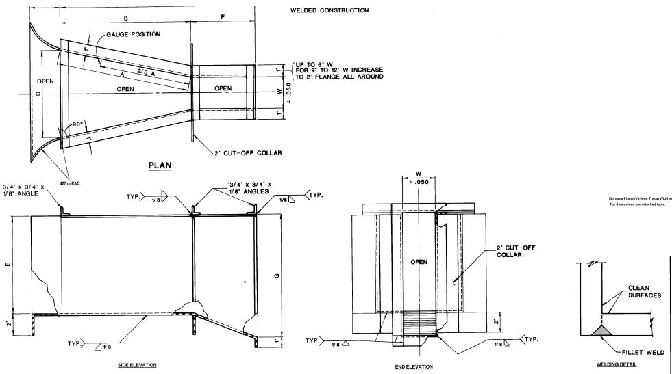
**Figure C-35. Various throat widths for the Montana flume.**
