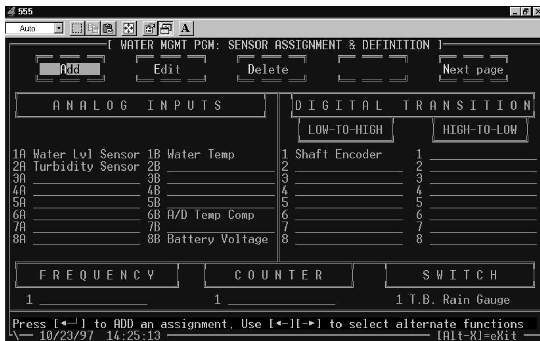
**Figure C-3. Programming screen showing types and allocation of sensors being used.**
