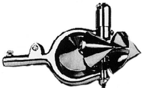
**Figure C-16. Price 622AA meter with retro-fit kit containing magnetic reed switch contact chamber.**
