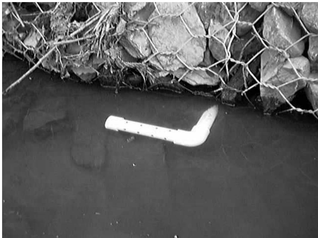
**Figure C-7. Static tube for intakes.**
