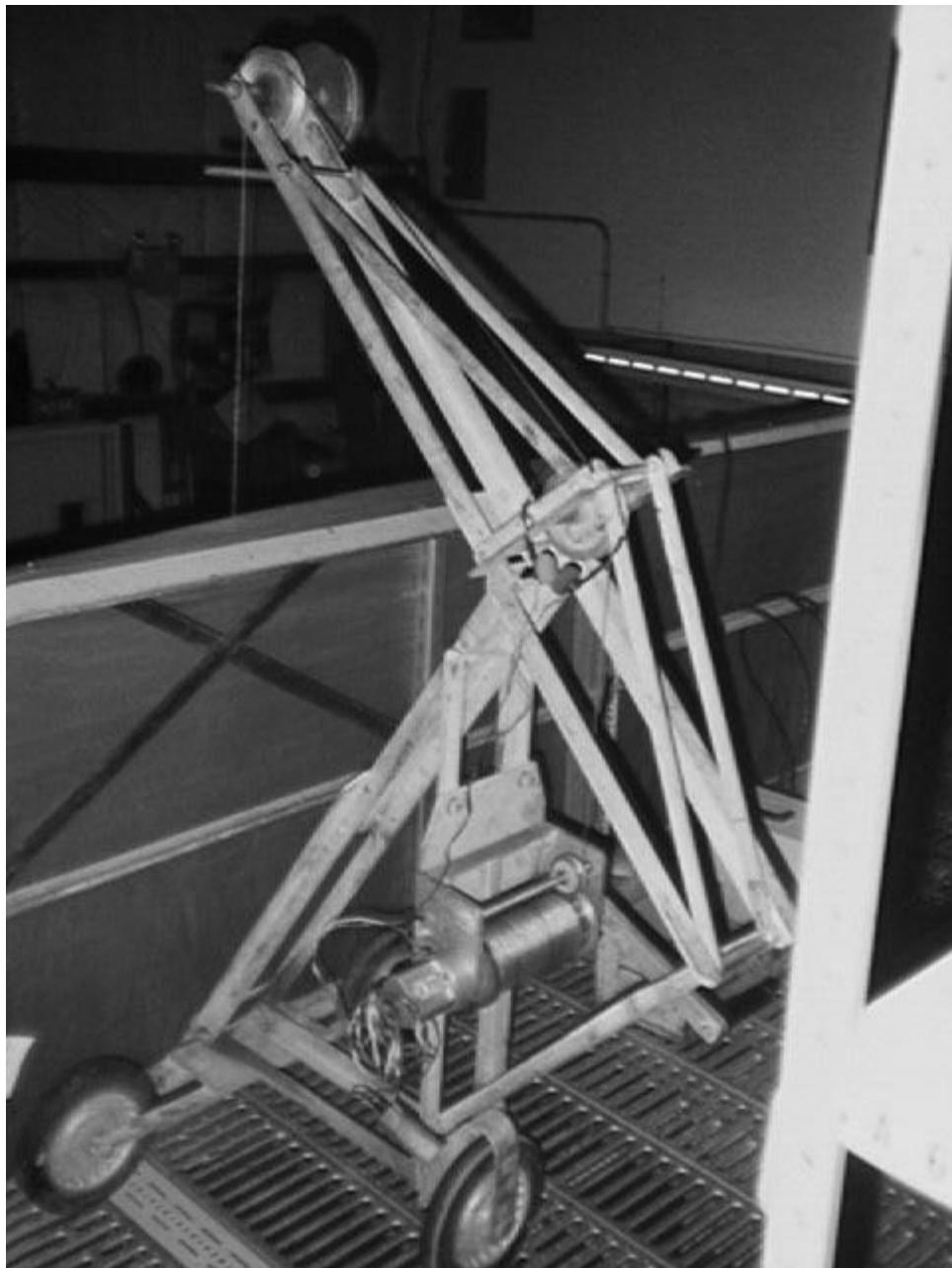
**Figure D-12. Three-wheeled bridge crane.**
