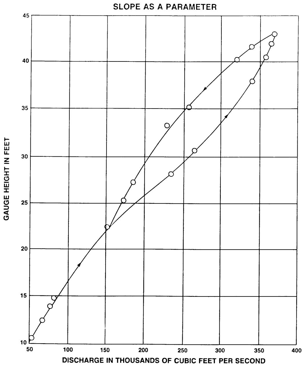
Figure F-6. Example of a stage-discharge loop.
