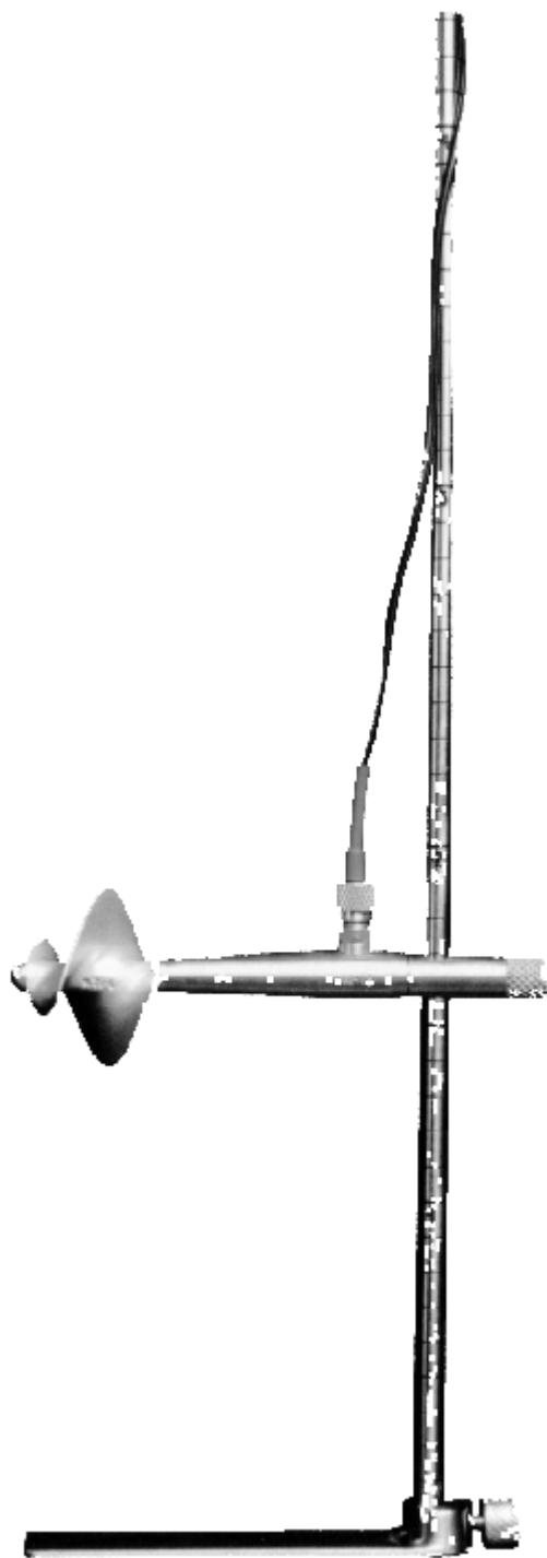
**Figure C-20. OTT C2 current meter, mounted on a 9-mm rod.**
