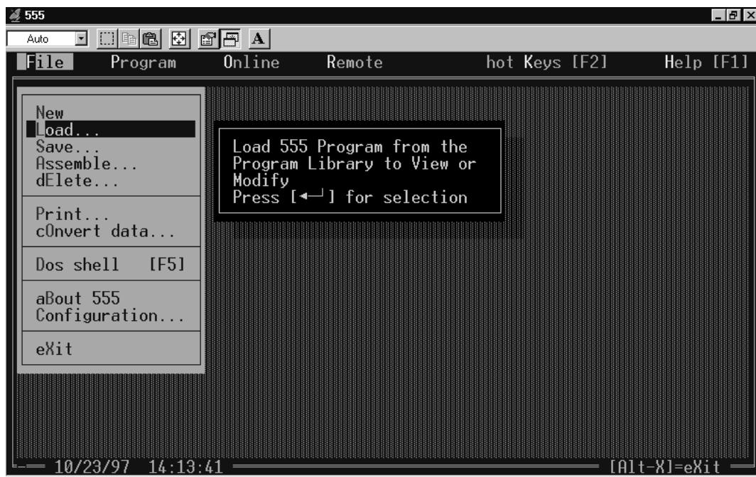
**Figure C-1. Typical menu-driven software package.**
