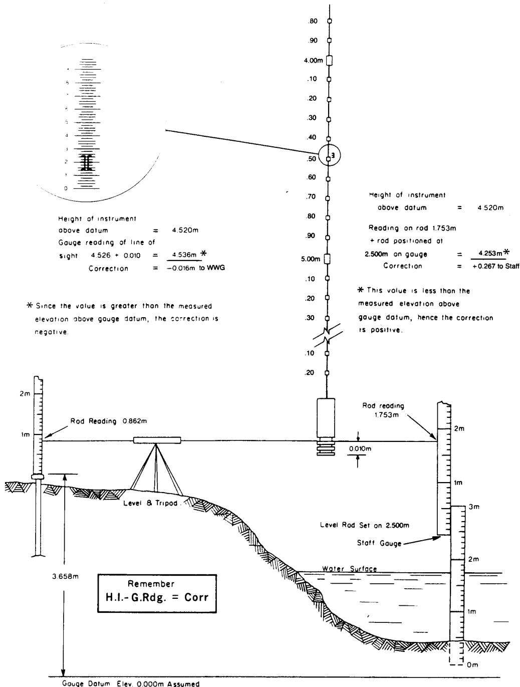
**Figure E-7. Gauge corrections and how they are derived.**
