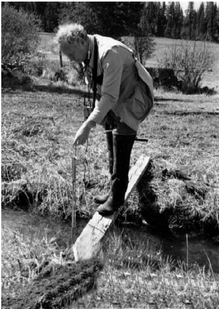
**Figure D-2. Ditch flow measurement using planks.**
