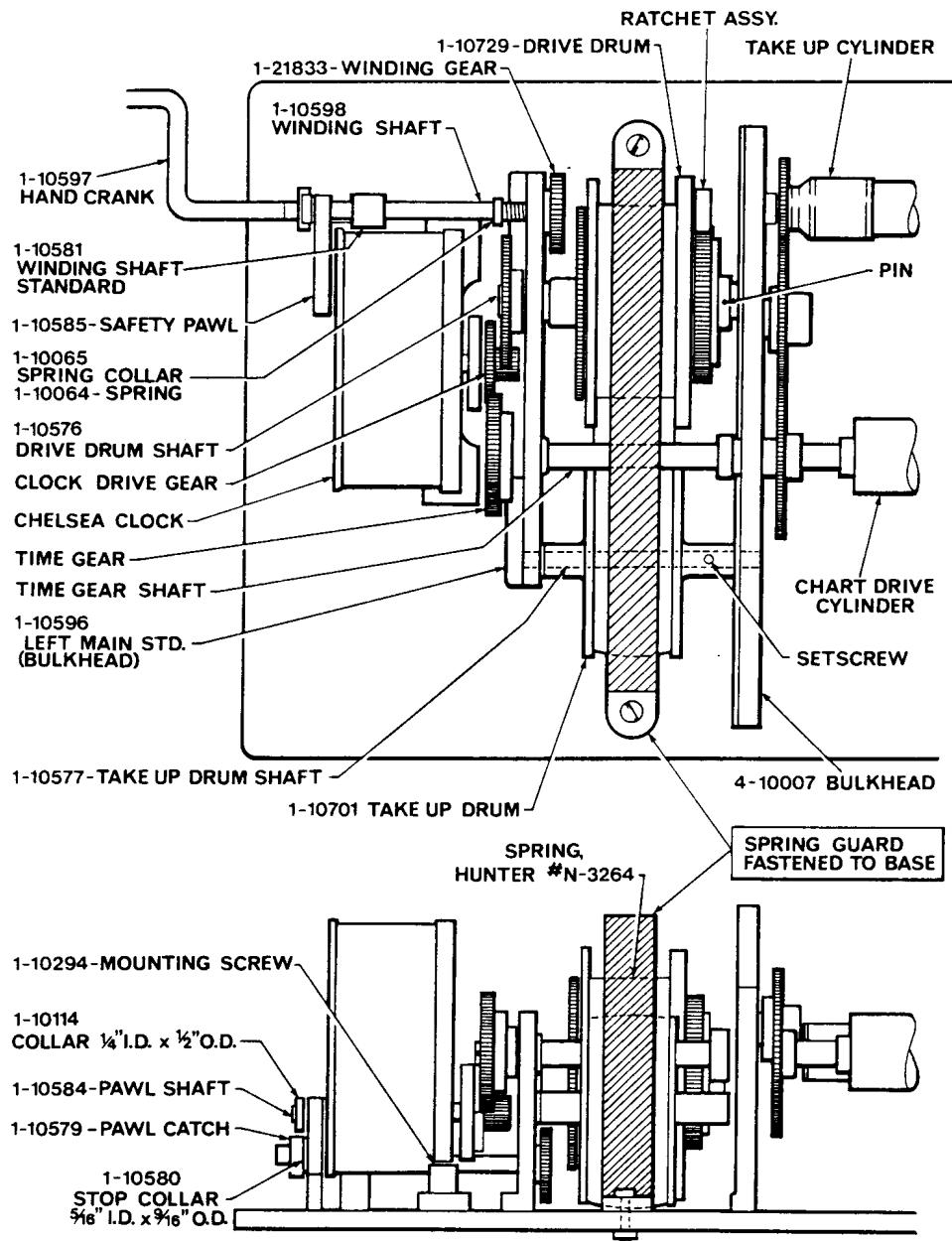
**Figure III-8. Negator spring drive**
