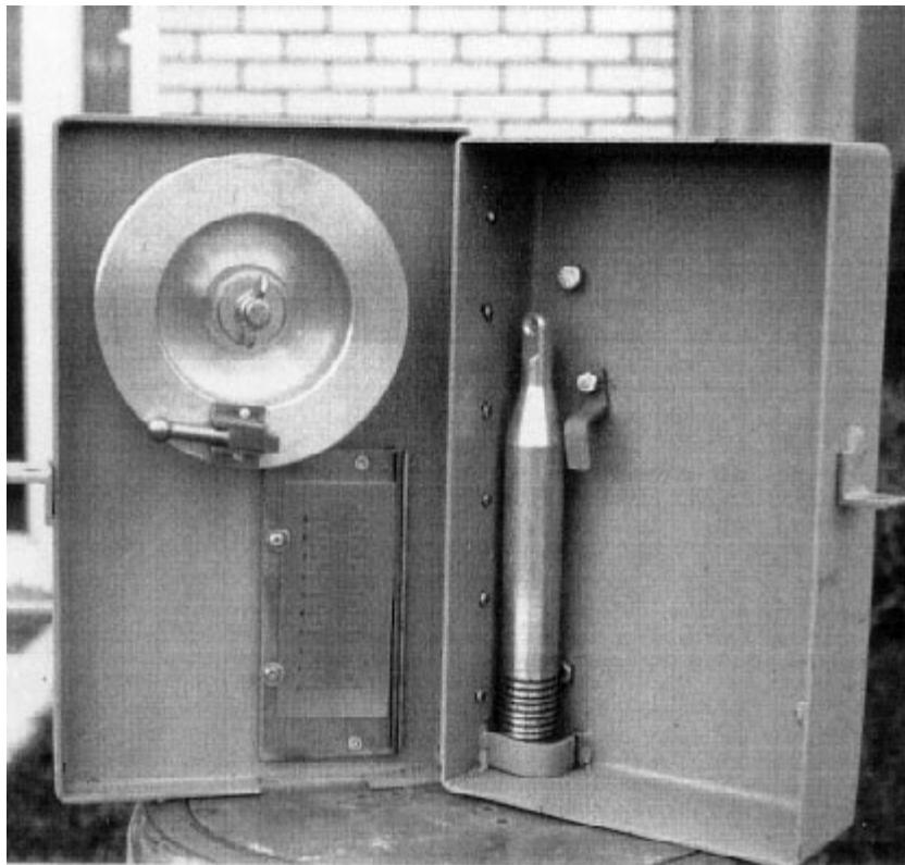
**Figure B-18. Wire-weight gauge with decimetre plate.**
