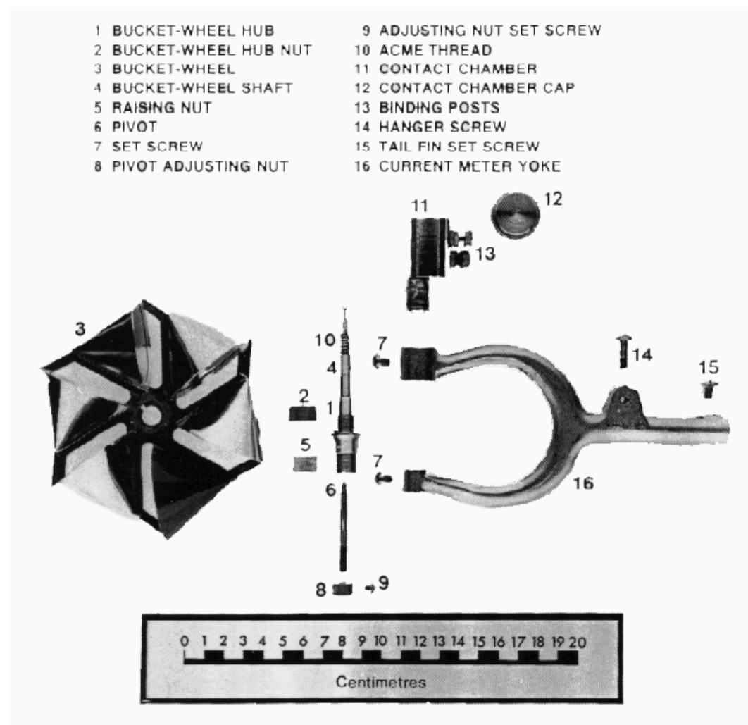
Figure C-14. Components of the Price 622AA current meter.
