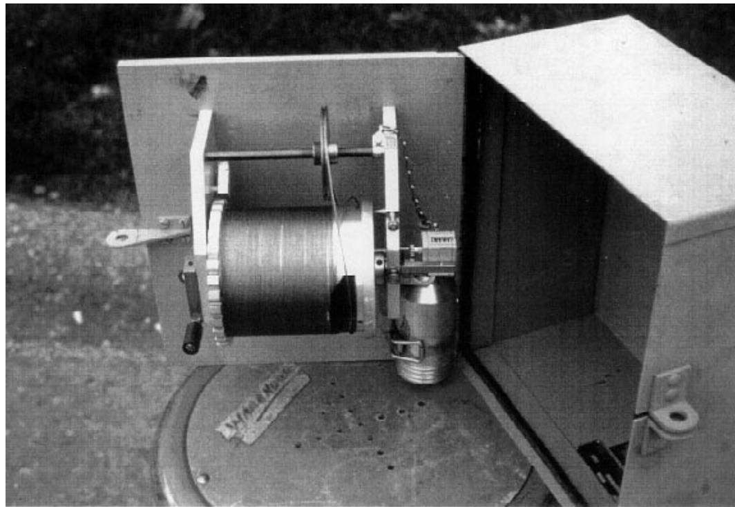
**Figure B-19. Non-Tagged wire-weight gauge.**
