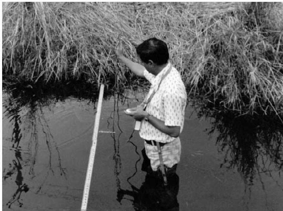
**Figure D-6. The technician is positioned downstream and to the side of the meter.**
