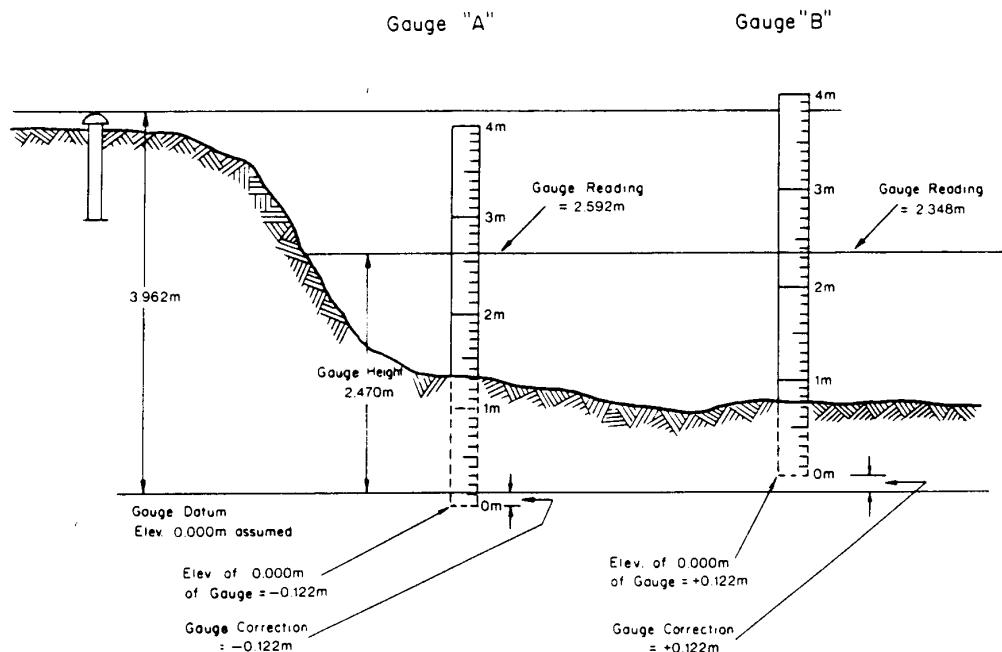
**Figure E-6c. Illustration of corrections to staff gauges.**
