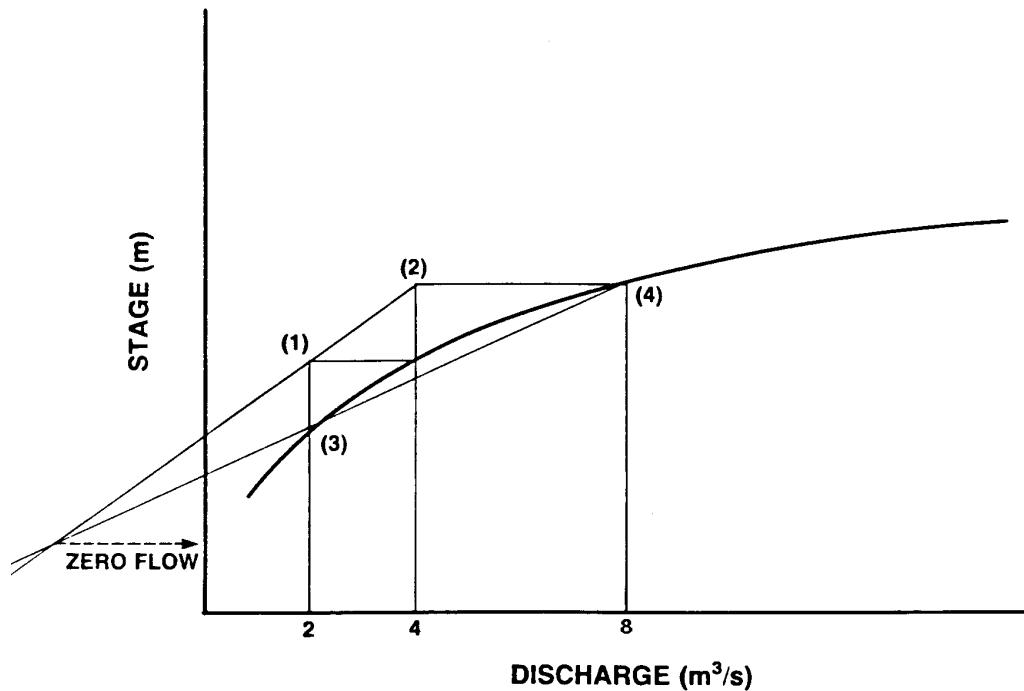
**Figure F-2. Graphical method for obtaining zero flow gauge height.**
