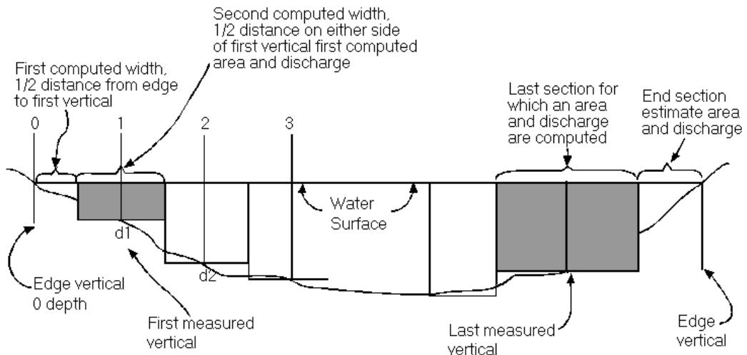
**Figure D-5. Mid-section method of discharge measurement.**
