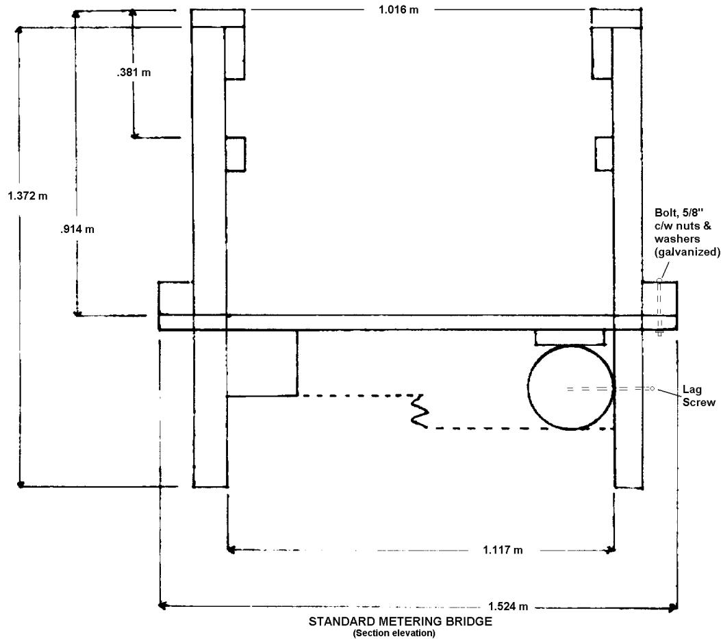
**Figure C-37. Section elevation of a standard metering bridge.**
