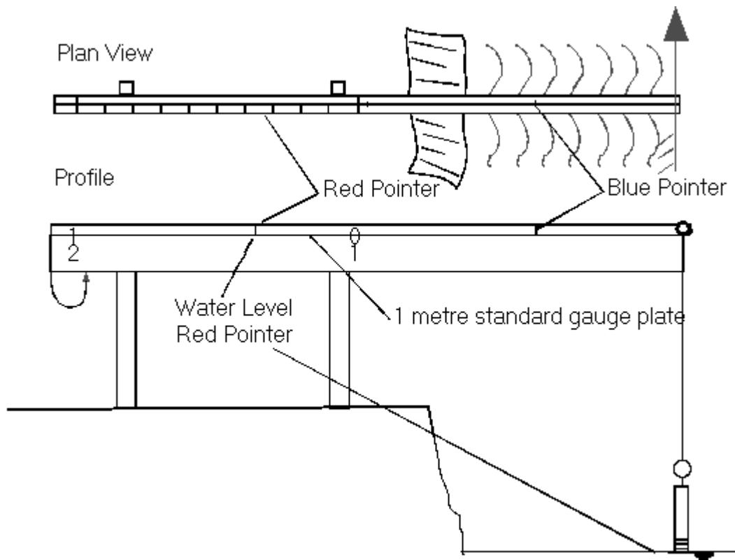
**Figure B-12.** Each meter, or part of meter, requires colour-coded tags and numeral plates. The spacing between the tag points must be exactly 1.000 m.
