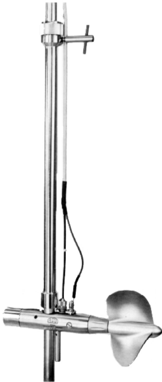
**Figure C-24. OTT C31 current meter fitted on a 20-mm rod, with relocating device.
