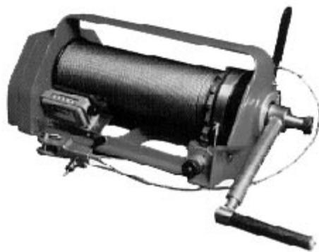
**Figure C-31.** San sounding reel, made in Australia.
