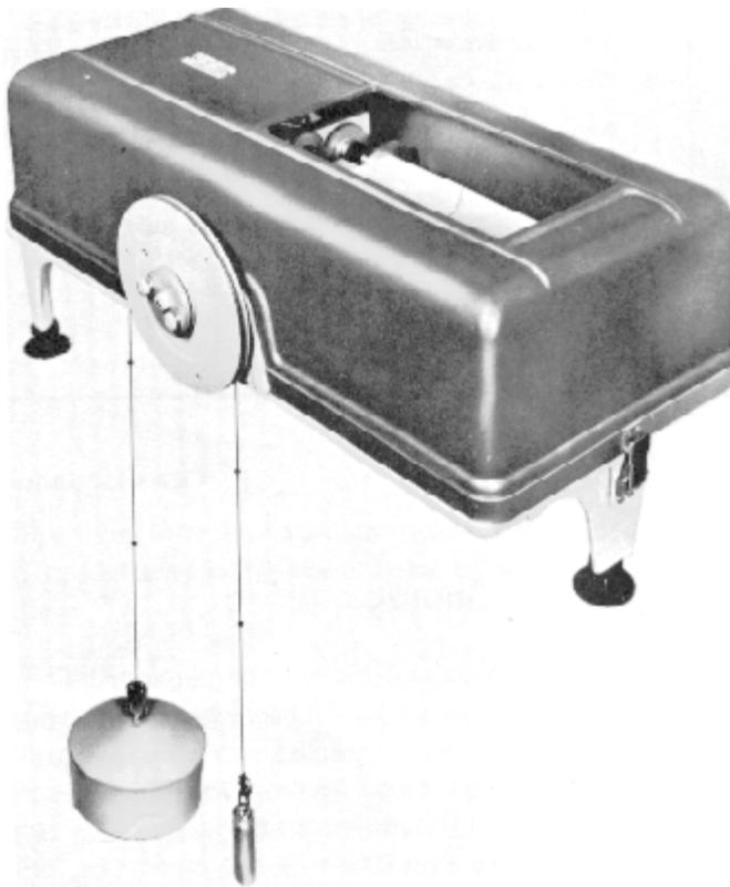
**Figure C-13. Stevens A-71 recorder with beaded float wire.**
