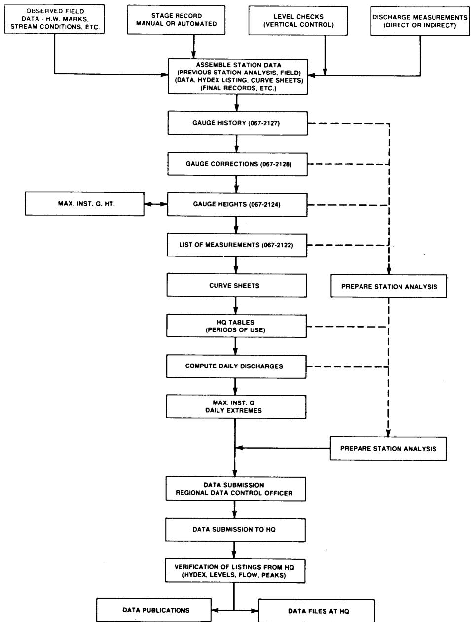
Figure F-5. Flowchart for manual computation of streamflow data.
