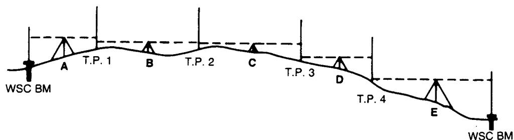
**Figure E-11. Differential leveling.**
