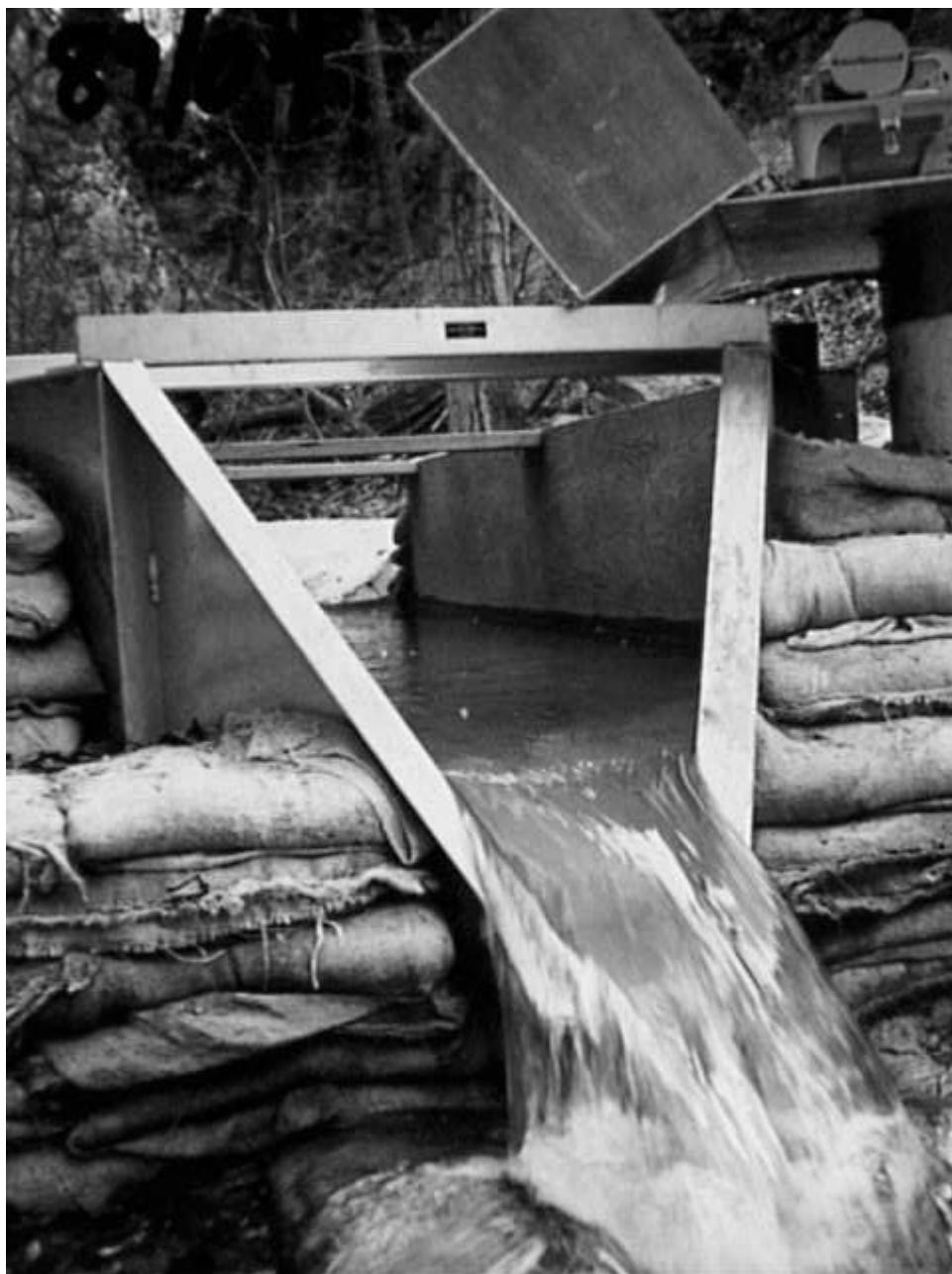
**Figure G-3. 2.5 foot H Flume set in concrete filled sacks. Cuisson Creek above
