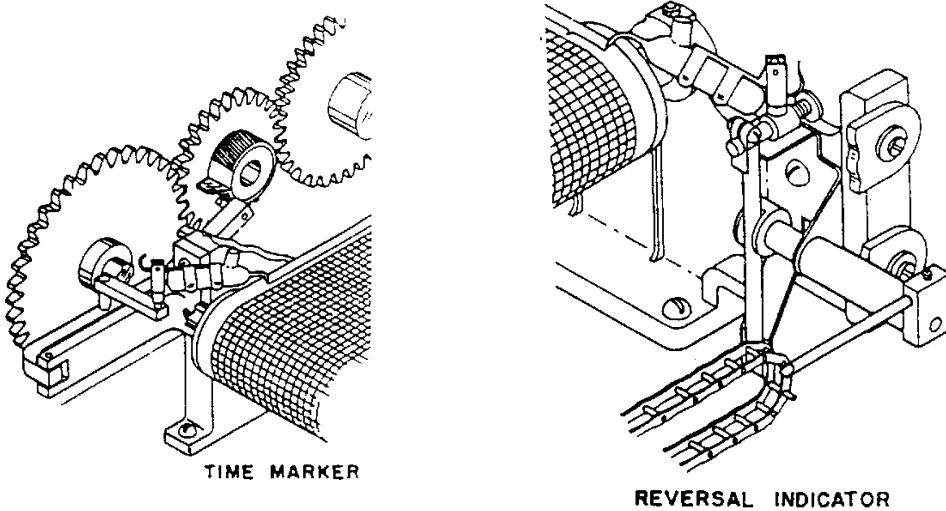
**Figure III-9. Recorder chart elapsed time marker**
