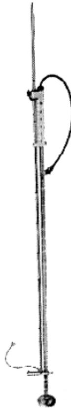
**Figure C-27. Top setting wading rod.**
