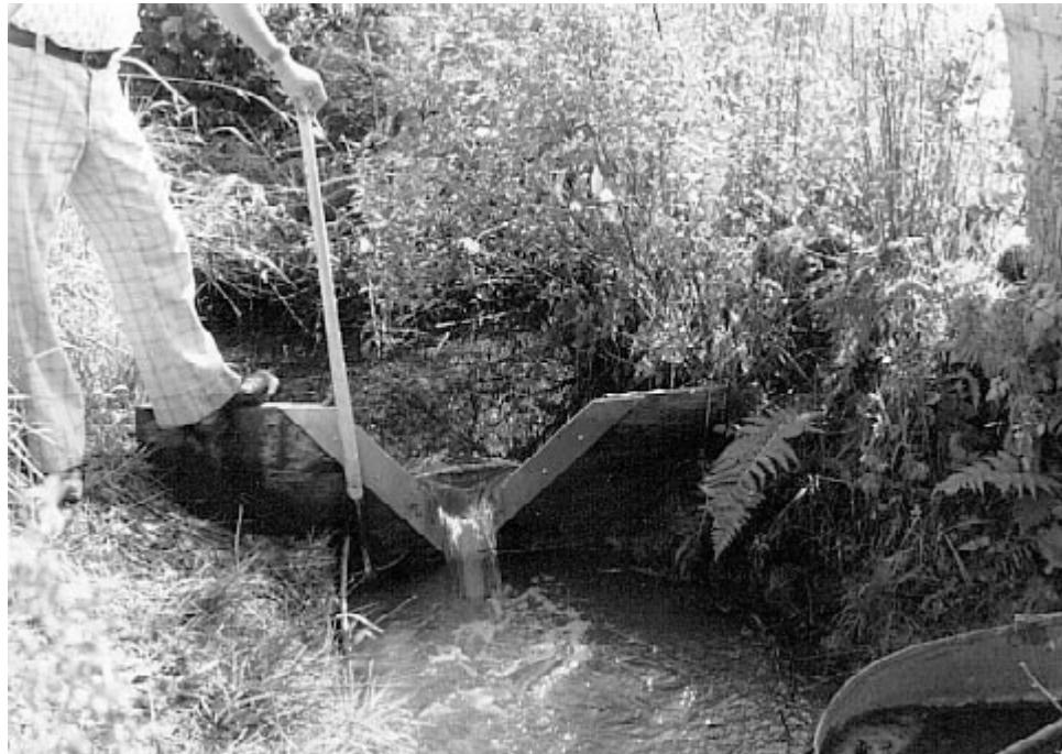
**Figure B-6. V-notch weir, portable installation.**
