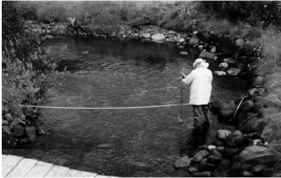
**Figure D-4. Conducting a discharge measurement with tagline across the wading section, Bridge Creek below Deka Creek.**
