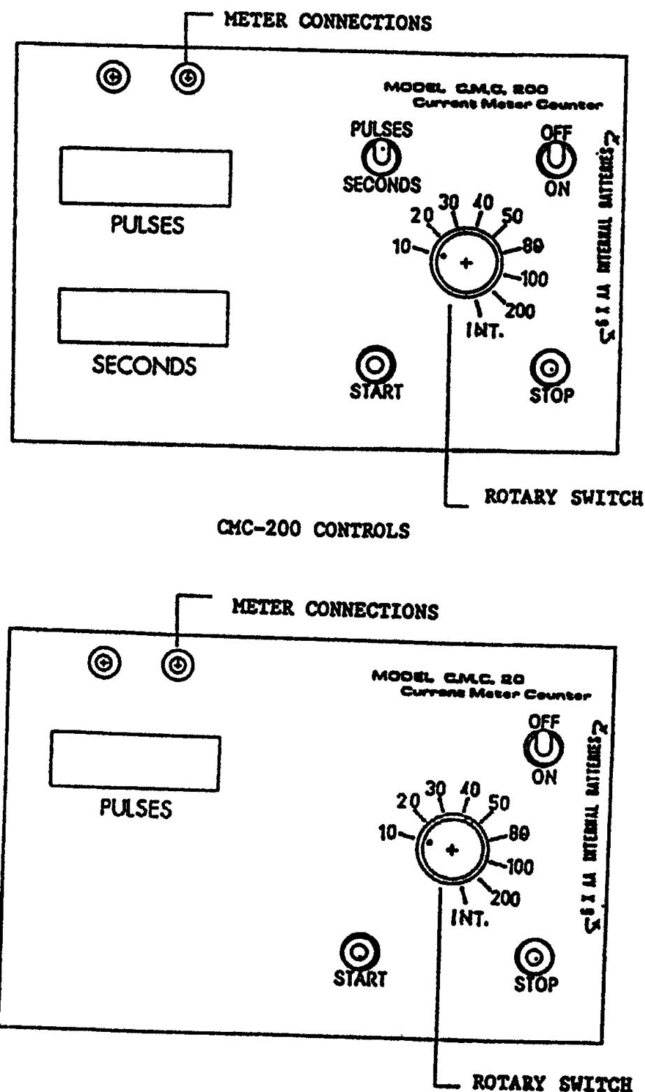
Figure C-26. Panel layout for the CMC-200 (top) and CMC-20 (bottom) counters.
